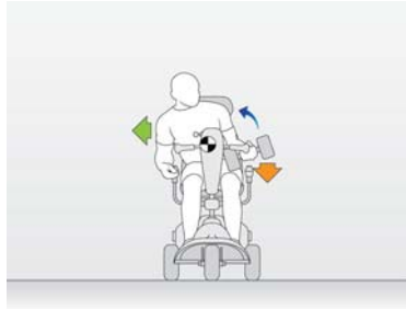
Correct lateral stability method
